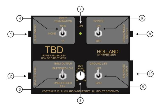
1. **Input-** This ¼" jack is the signal input. Plug in your guitar or keyboard here. The TBD circuitry places virtually no load on the input source with the input
